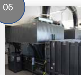
Unique Horizontal Motorized waste/air separation unit IMWS™
